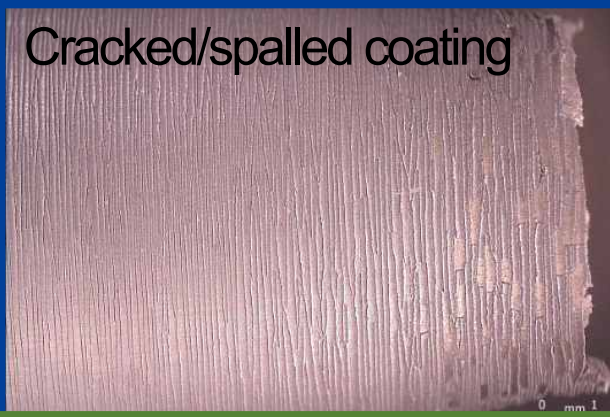
Cracked/non-dense coating
